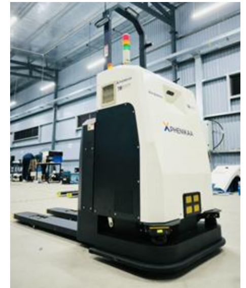
AMR Pallet Mover - robots help automation at Samsung Factory
